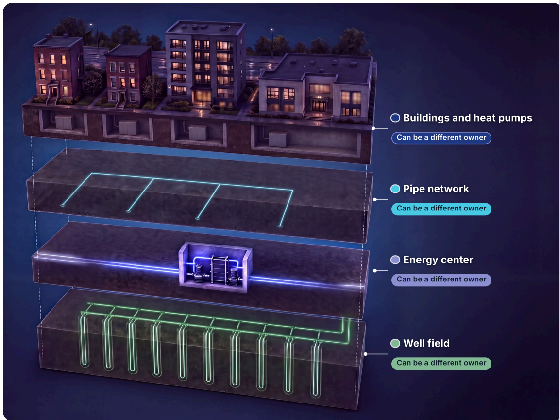
Figure 2. One network, four layers: buildings with their heat pumps, the pipe network, the energy center and the well field. Each layer can have a different owner. The federal credit goes to the party that owns the ground loop and at least one connected heat pump (Treasury T.D. 10015 2 ), so the way the layers are split decides who can claim it. Gaiergy illustration.
