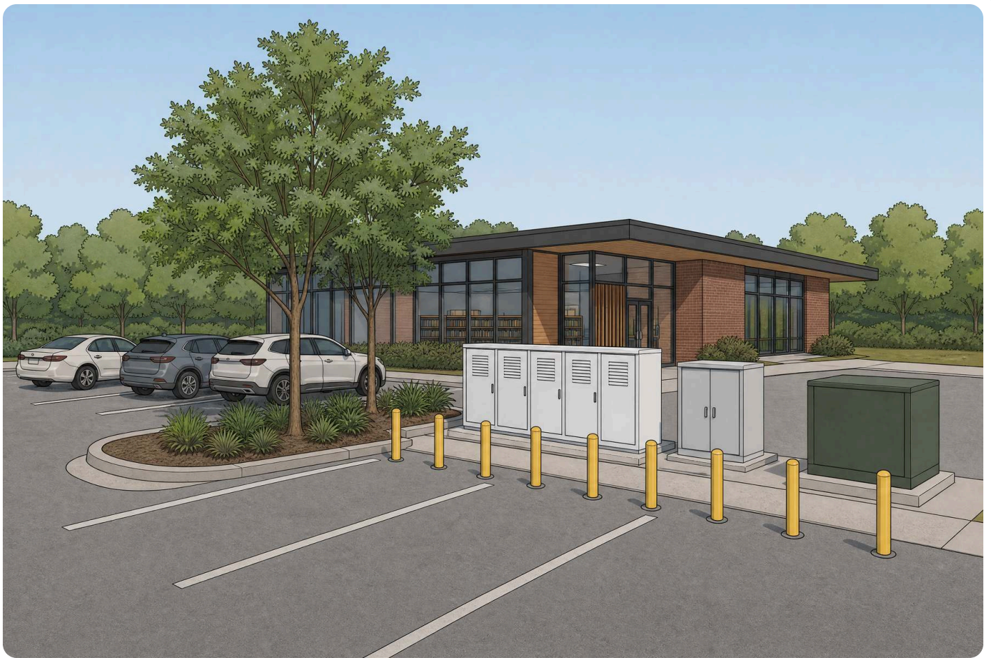
Figure 10. Building-scale cabinets in a parking lot, with vehicle barriers and clear space. Illustration, Gaiergy.
