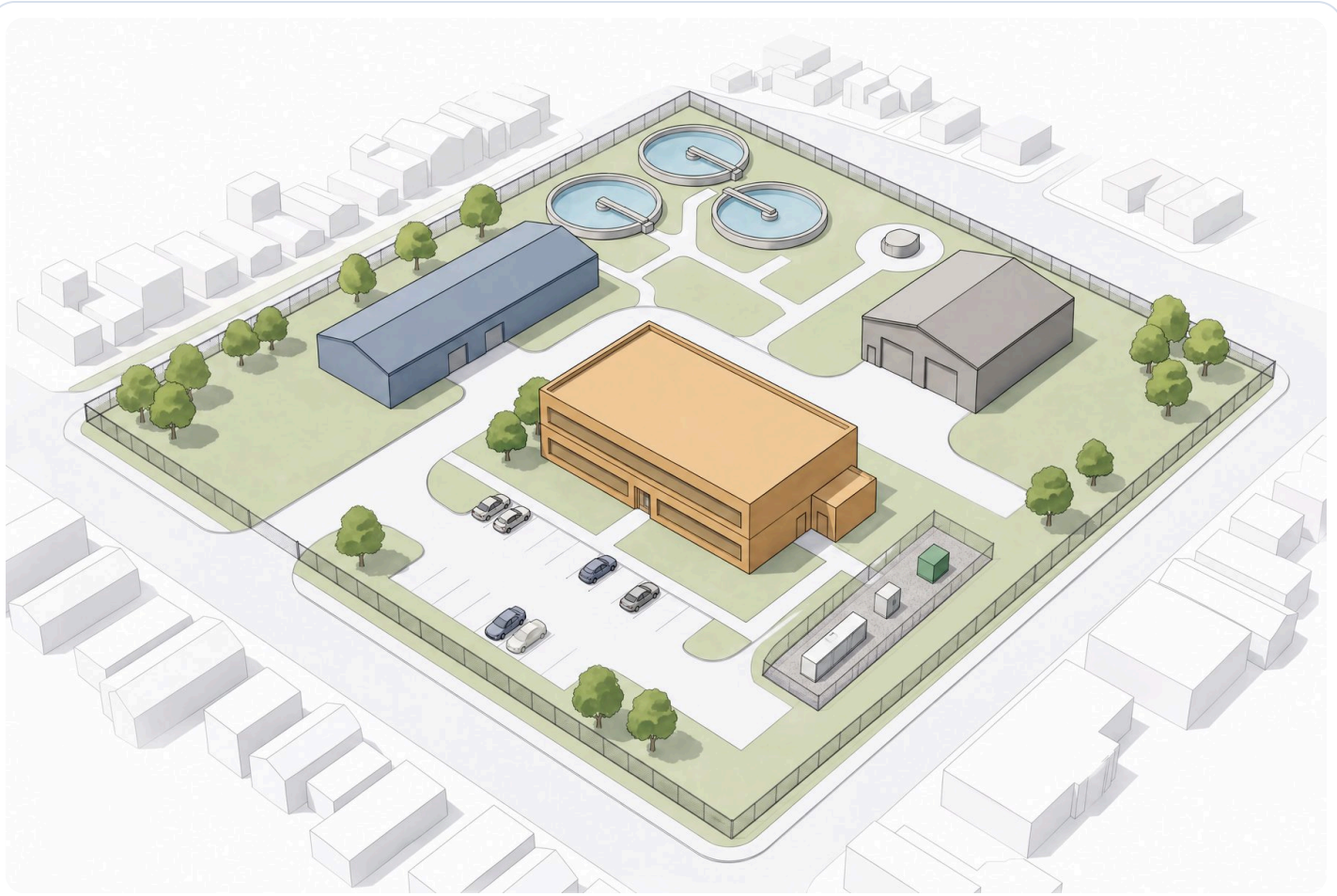
Figure 13. A city campus: the battery sits next to the plant's electric service, where it can cut the plant's peak. Illustration, Gaiergy.
