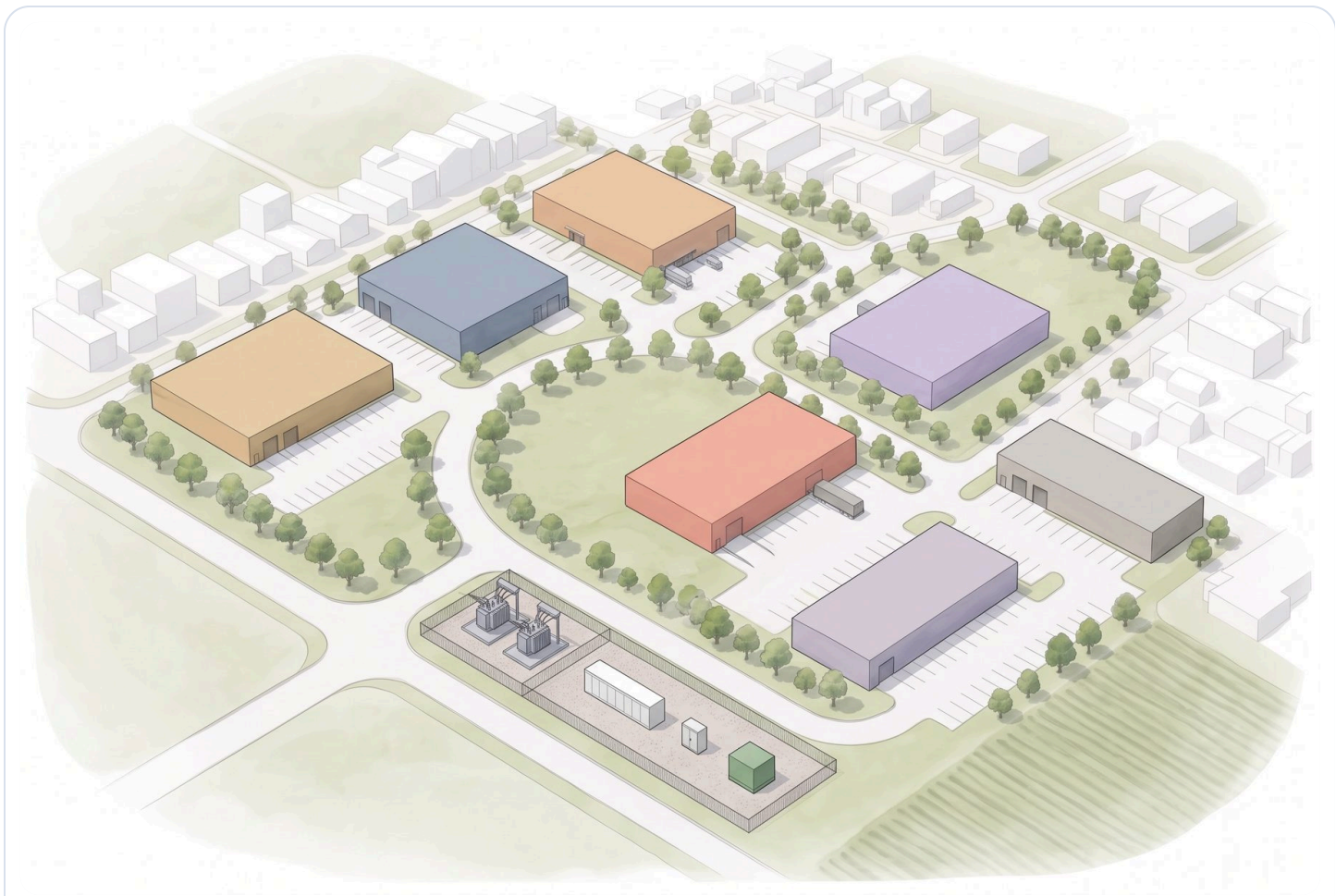
Figure 54. An industrial park shares one battery yard next to its own substation. Illustration, Gaiergy.
